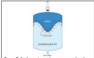
**figure 2.** As the water and pressure reaches its maximum, the diaphragm flexes against the air cushion (air is compressible) to allow for increased water expansion.
